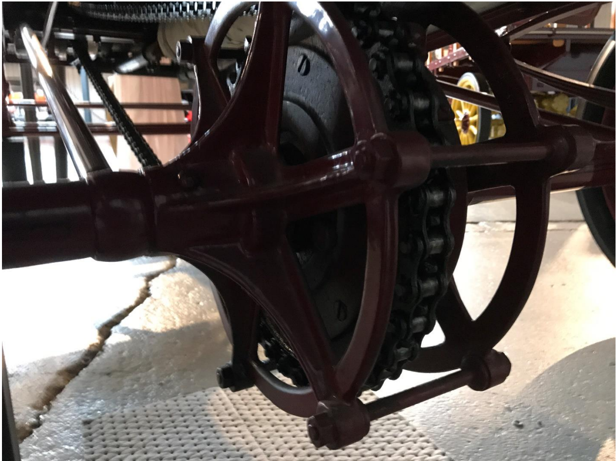
A sprocket gear differential mounted on an Franklin CDA at the Northeast Classic Car Museum, Norwich, N.Y. (Photo by the author)
